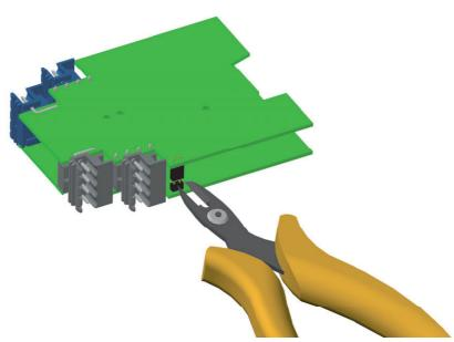
Cut both pins of the connector to open the wiring between the terminals, using a wire cutter
